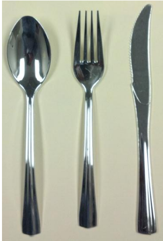
Photograph 1 Aluminum-coated product as- purchased before dishwashing.
