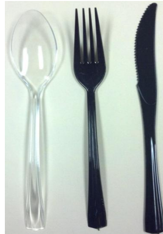
Photograph 2 Aluminum-coated product after dishwashing. As shown, all coating has been washed off and parts show their original “unmetallized” appearance (i.e., clear or black).
