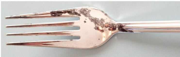
Photograph 3 Aluminum coated fork subjected to spaghetti sauce for an hour. The coating flaked off in several locations on the fork head.
