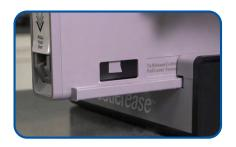
Start by sliding the tower partially or fully out of base (do NOT place on side or tip upside down, keep the tower upright).
